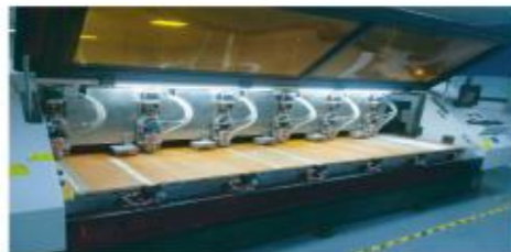
CNC machine CNC drilling machine maintenance
